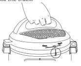
**02** Turn the lid clockwise until the **▼** on the lid aligns with the middle of the control panel.
